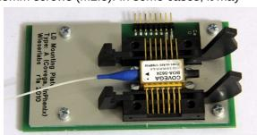
help to first put the screws through the butterfly package and then put the package with the screws on the mounting plate.
