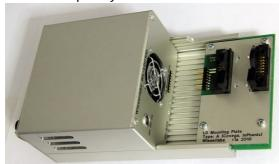
3. Open the butterfly mount and insert the laser diode (SOA, BOA) in butterfly package. Ensure the pin 1 is on the correct side. Pin 1 is marked on the mounting plate and usually also on the butterfly mount. (Note: There are different mounting plates for different pinouts.) Put the 4 fixing screws through the holes of the butterfly package and the mounting plate. The screws supplied with the LDC10D are standard metric 2.5mm screws (M2.5). In some cases, it may
