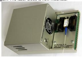
Note: The screws ensure that the butterfly package has good thermal contact with the aluminum LD mounting plate for heat sinking.
