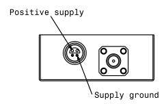
Supply connector (front view). The case is electically connected to ground.
