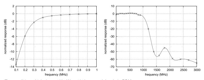
Test conditions: Light input 100  $\mu\mathrm{W}$  at 1310 nm, modulated via EOM.
