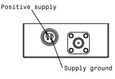
Supply connector (front view). The case is electically connected to ground.
